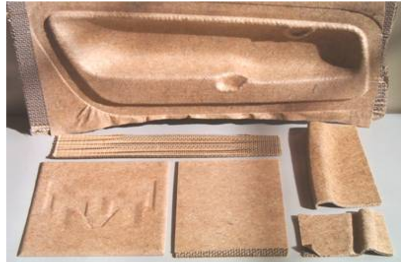
TorHex PP/natural fibre door panel
